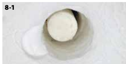
Figure 8-1: As shown in the figure, press ceramics are increasingly accumulated on the surface of the press-fitting plunger if the attached press ceramics are left unremoved. Therefore, press ceramics attached to this part should periodically be scraped off.
