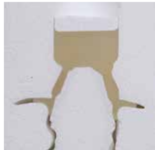
Figure 5-6: Press molding in an investment mold.
