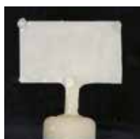
Figure 3-1: The length of each sprue in the left and right figures is 3 mm and 5 mm, respectively. The Ready Casting Wax R25 was used for both sprues and 0.46 mm-thick sheet waxes for press molding.
