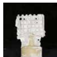
Figure 3-1: The length of each sprue in the left and right figures is 3 mm and 5 mm, respectively. The Ready Casting Wax R25 was used for both sprues and 0.46 mm-thick sheet waxes for press molding.
