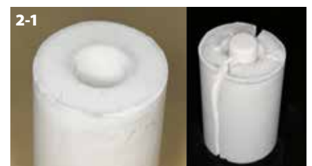
Figure 2-1: Left: Cracks after burnout. When the ring is placed in the ring furnace at 500°C and then the temperature is raised to 900°C, the ring may crack as shown in the figure. Right: As shown in the figure, the investment having a decreased compressive strength may fail when pressed.
