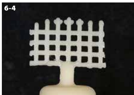
Figure 6-4: Ideally pressed condition into mesh pattern. (The wax pattern of GEO retention grid, fine from Renfert and the sprue of R25 are used.)
