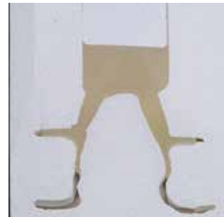
Figure 5-6: Press molding in an investment mold.
